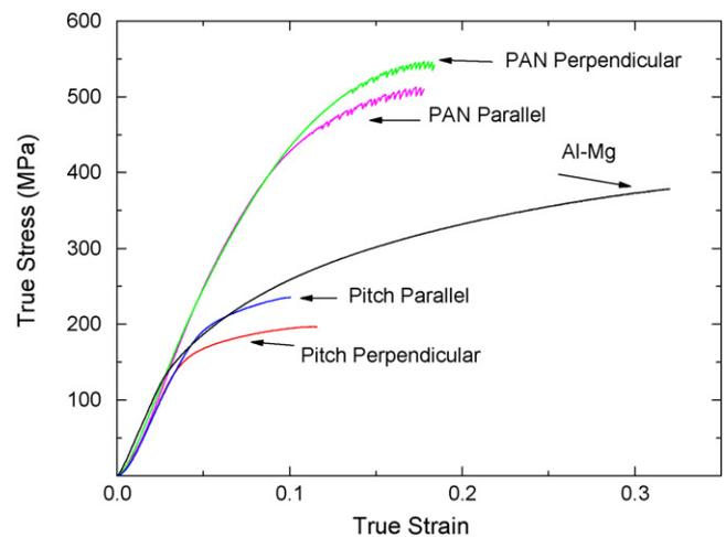
Fig. 2. Typical stress-strain curves of cylindrical specimens under quasi-static compression ( $\sim 10^{-3} \text{ s}^{-1}$ ) for Al-Mg and two composites (PAN or pitch fibers parallel or perpendicular to loading).
