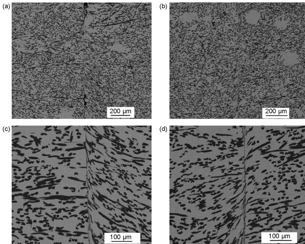
Fig. 7. SEM micrographs exhibiting the shear zone and plastic flow pattern in a  $C_{\text{Pitch}}/\text{Al-Mg}$  specimen: (a) low magnification of shear zone (left hand side of the sheared sample); (b) low magnification of shear zone (right hand side); (c) high magnification of shear zone (left hand side); (d) high magnification of shear zone (right hand side).
