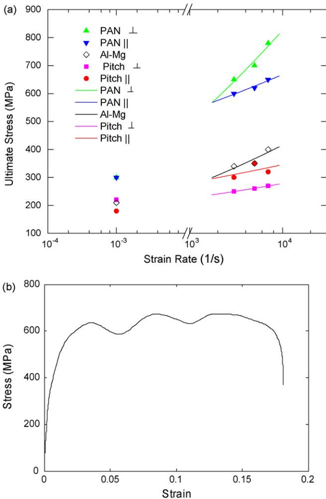
Fig. 4. (a) Experimental data (all symbols) and fitted curves (only for the data from high-strain rate deformation) of all materials and (b) stress–strain curve of a  $C_{\text{PAN}}/\text{Al-Mg}$  composite specimen at  $7000 \text{ s}^{-1}$  deformation.
