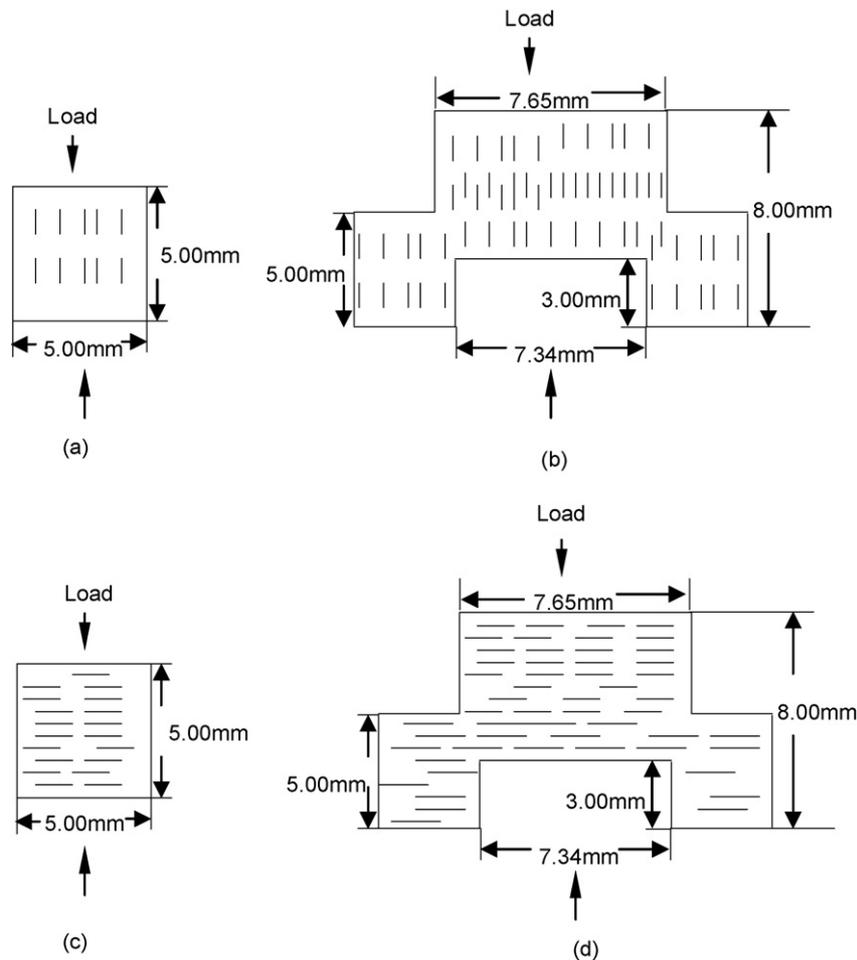
Fig. 1. Geometry of cylindrical and hat-shaped specimens: (a and b) fibers oriented parallel (||) to loading direction and (c and d) fibers perpendicular ( $\perp$ ) to loading direction.
